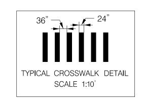
NOTE: START CROSSWALK MARKINGS IN THE CENTER OF LANES. SPACE BETWEEN MARKINGS SHOULD BE PLACED IN WHEEL TRACKS OF EACH LANE. DISTANCE CAN BE ADJUSTED TO AVOID WHEEL PATHS.
